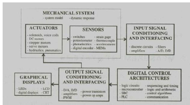
Figure 2: Block Diagram of Mechatronic System
