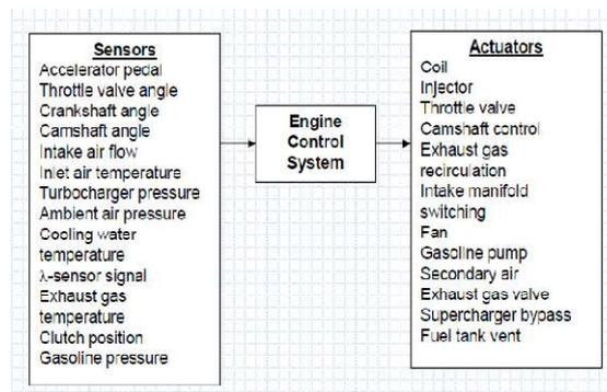
**Figure 11: Mechatronic Elements of Engine Control System**
