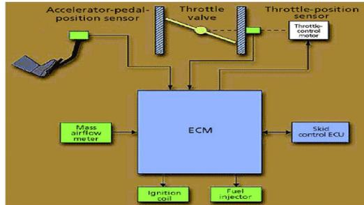
**Figure 15: Throttle Position Sensor**
