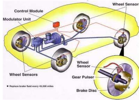
**Figure 7: Antilock Brake System (ABS)**
