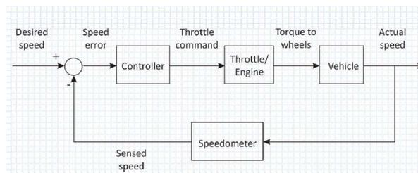
**Figure 9: Cruise Control System in Car**
