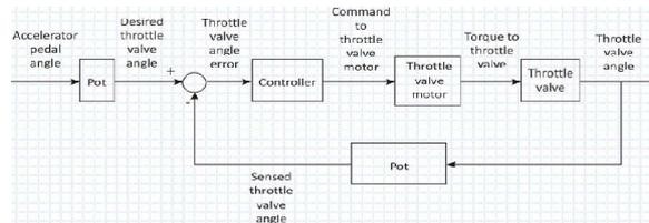
**Figure 16: Throttle-by-Wire Control System**
