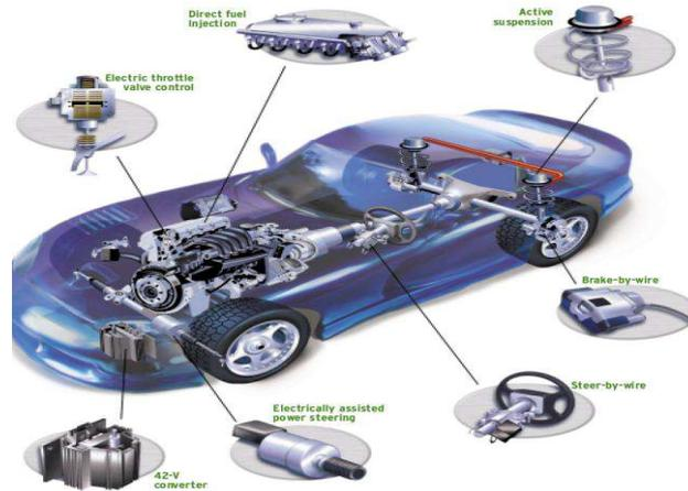
Figure 5: Mechatronic Systems in Automobile
