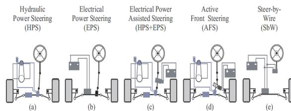
**Figure 4: Mechatronic Steering Systems: (a) Conventional Hydraulic Power Steering (HPS) (Since about 1945); (b) Electrical Power Steering (EPS) for Smaller Cars (1996); (c) Electrical Power Assisted Steering (HPS+EPS) for Larger Cars; (d) Active Front Steering (AFS): Additional Wheel Angles Generated by a Planetary Gear and a DC motor (2003); (e) Steer-by-Wire (SbW)**
